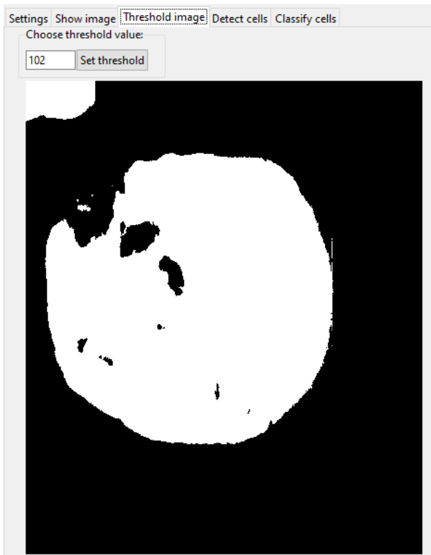
Figure 4.35: Threshold image. This tab provides the option to enhance the image contrast by thresholding (disabled for light and fluorescence microscopy)
