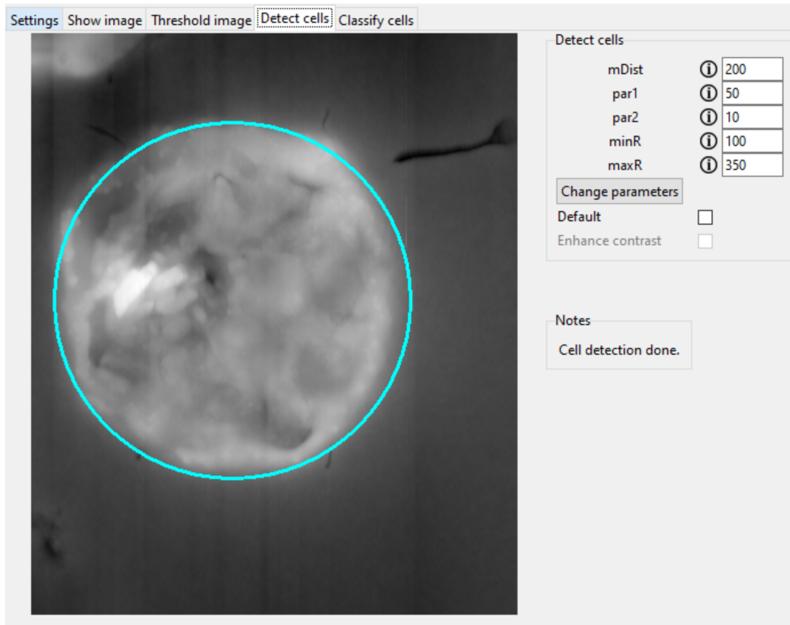
Figure 4.36: Detect cells. RBCs in the images are detected by the cell detection algorithm. To fine-tune, the algorithm offers the possibility to enhance the image and to set the parameters for the detection manually.
